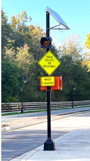
Signs with flashing beacons that activate when rail crossing is blocked are effective and affordable alternatives to dynamic message signs.
