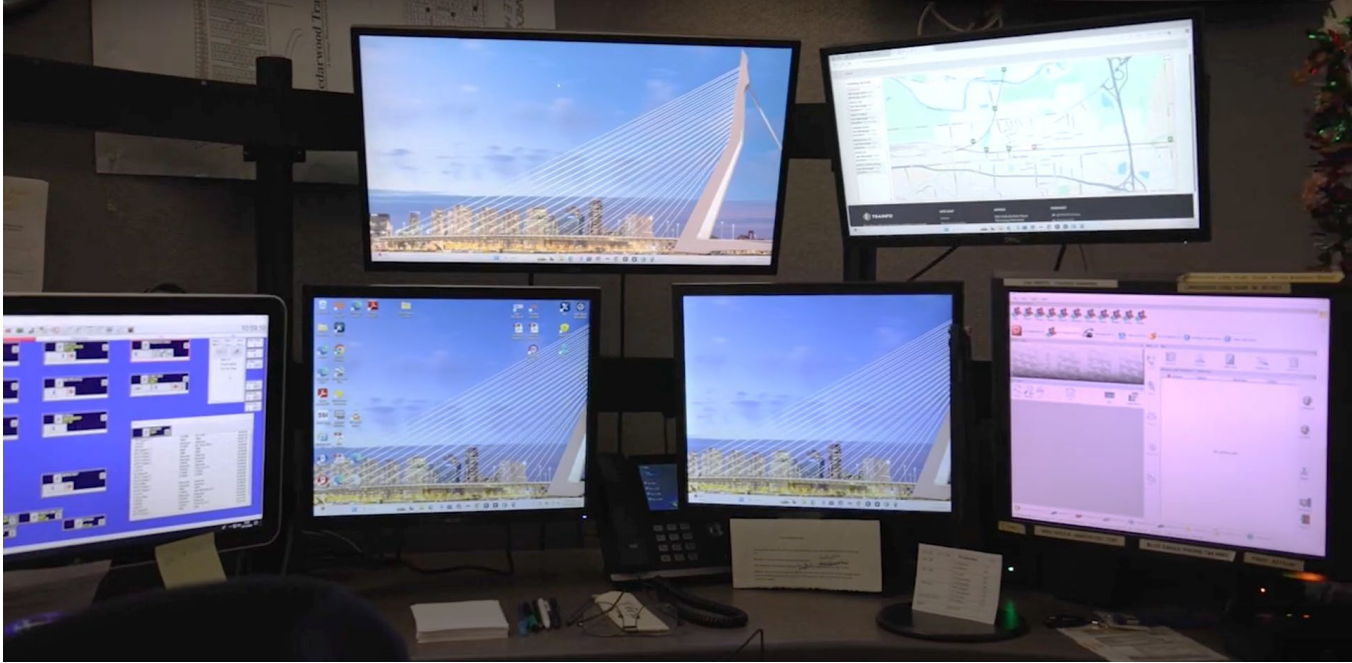
Real-time rail crossing information is provided to emergency dispatchers (top left screen). This enables dispatchers to select units and routes to emergencies that avoid delays due to blocked crossings.
